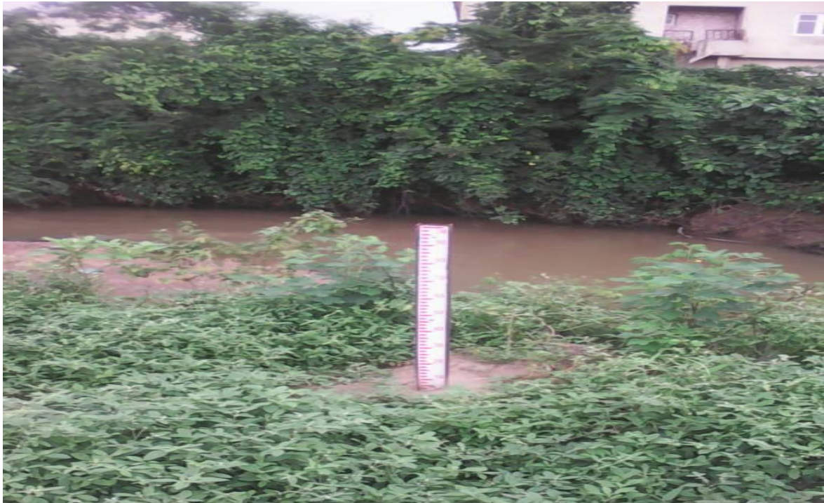
Figure 5. 21: Sample of Installed river gauge by SESA Consultant at communities within the river channels –at kudeti, Ogbere tioya, Akinwunmi, Ogundipe kumapayi.
